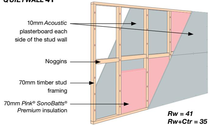
Note: 90mm studs will increase the acoustic performance of the wall system. Figures calculated using Insul insulation prediction software.
