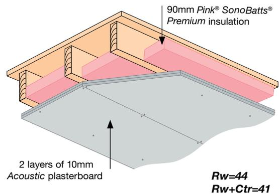
Note: System based on standard timber floor joists. Figures calculated using Insul insulation prediction software.
